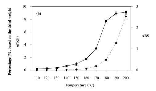
**Fig. 1.** The effect of temperature on the hydrolysis of konjac powder: (a) solid loss (■, solid line), total carbohydrates (♦, dotted line), reducing sugars (♠, solid line), final pH (●, dotted line), and protein (■, dotted line), and (b) 5-HMF (♦, dotted line) and UV absorbance level (■, solid line) of the hydrolyzed products (15 min, 0.05 M HCl, 10:1 of ratio of reaction volume to konjac powder mass).
