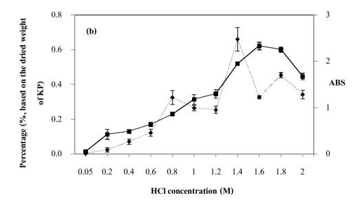
Fig. 2. The effect of HCl concentration on the hydrolysis of konjac powder: (a) solid loss (■, solid line), total carbohydrates (♠, dotted line), reducing sugars (♠, solid line), and protein (♠, dotted line), and (b) 5-HMF (♠, dotted line), and UV absorbance level of HP (■, solid line) (110 °C, 15 min, 10:1 of ratio of reaction volume to konjac powder mass).
