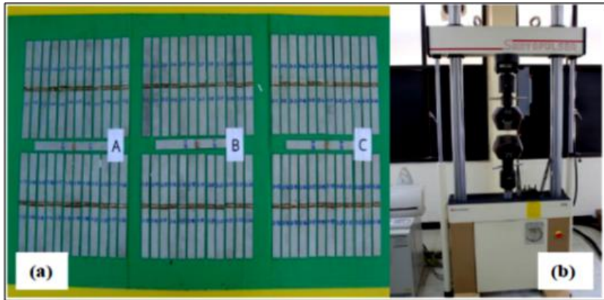
Fig. 6 TSS test specimens (a) and Universal testing machine.(b)
