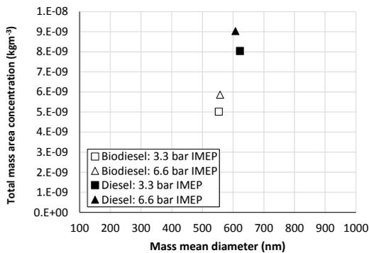
**Fig. 13** Relationship between total particle mass and mass mean diameter
