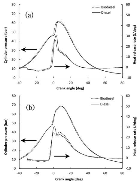
**Fig. 2.** In-cylinder pressure and heat release rate at 1,700 rpm (a) 3.3 bar IMEP and (b) 6.6 bar IMEP
