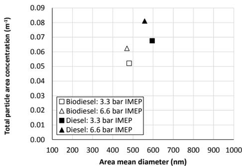
**Fig. 11** Relationship between total particle area and area mean diameter
