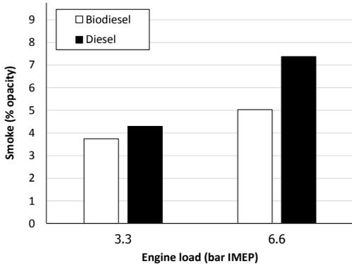
Fig. 7. The effects of engine load on smoke
