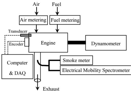
Fig. 1. Schematic diagram of engine test rig
