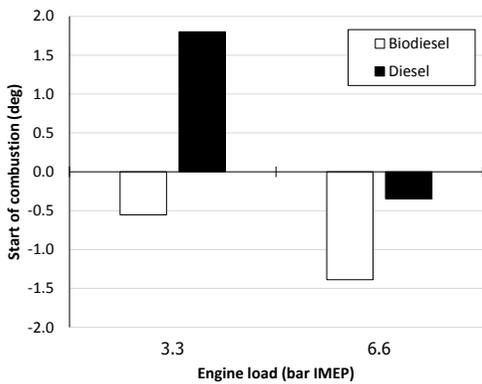
Fig. 3. The start of combustion for diesel and biodiesel
