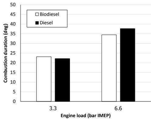
Fig. 4. Combustion duration
